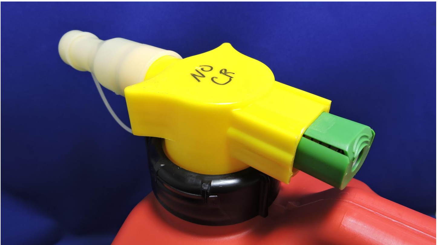
Photo #7 – View of Portable Fuel Container with Non-Child Resistant Push Button Feature for Screening Test
