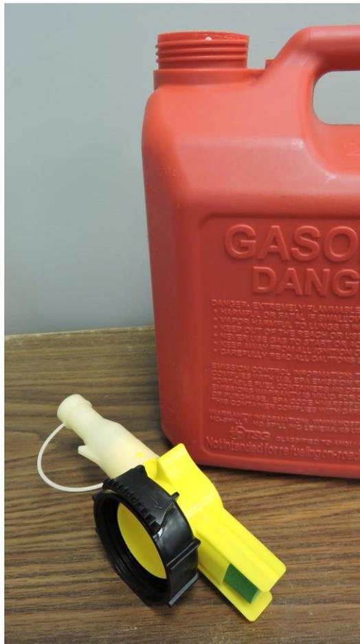
Photo #3 – View of Collar removed from the Portable Fuel Container
