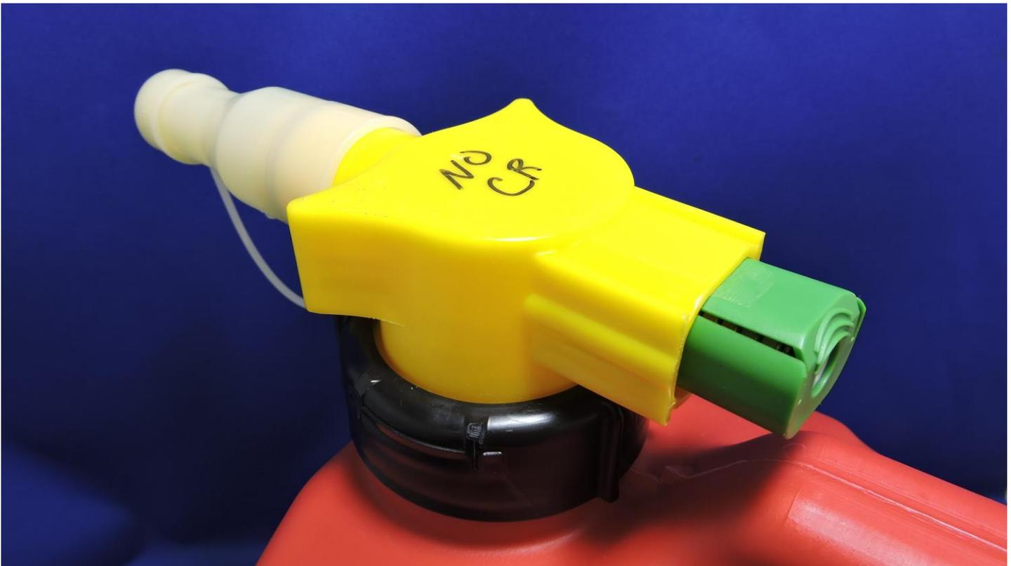
Photo #4 – View of Portable Fuel Container with Non-Child Resistant Collar for Screening Test
